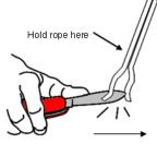
Slice rope from rear to front of cutting edge, cutting away from the body
